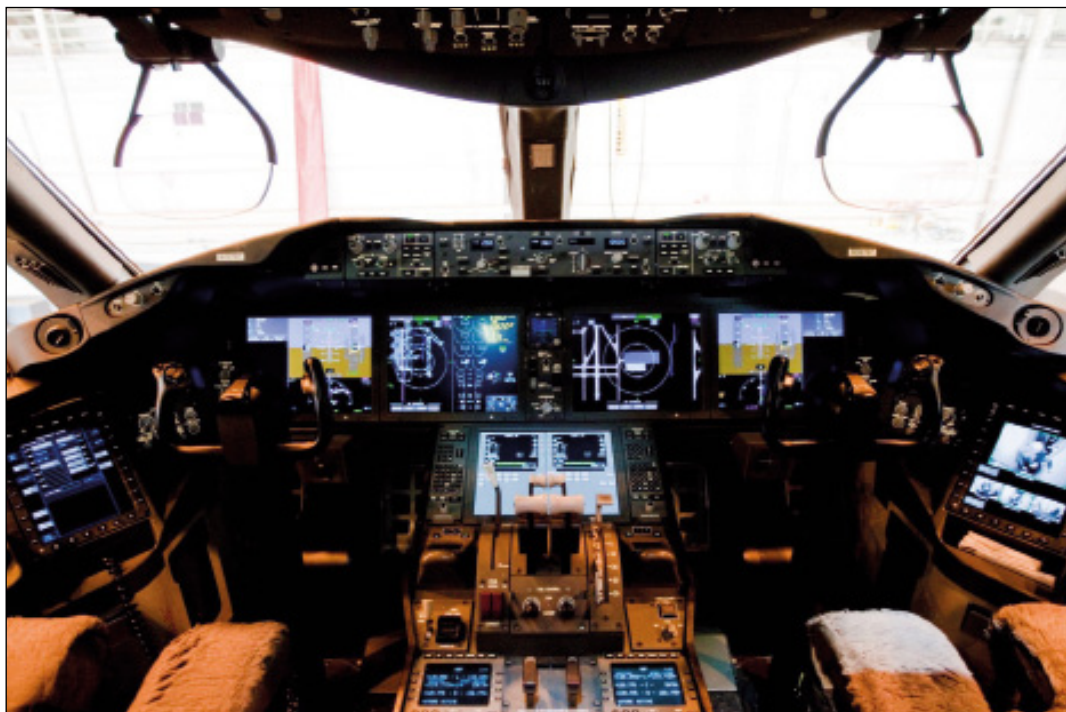
Fig. 1 - This cockpit from the B787 (The Dreamliner) is the largest commercial airliner recently placed in regular commercial traffic. Its cockpit is highly automated and largely managed by computerized commands.
